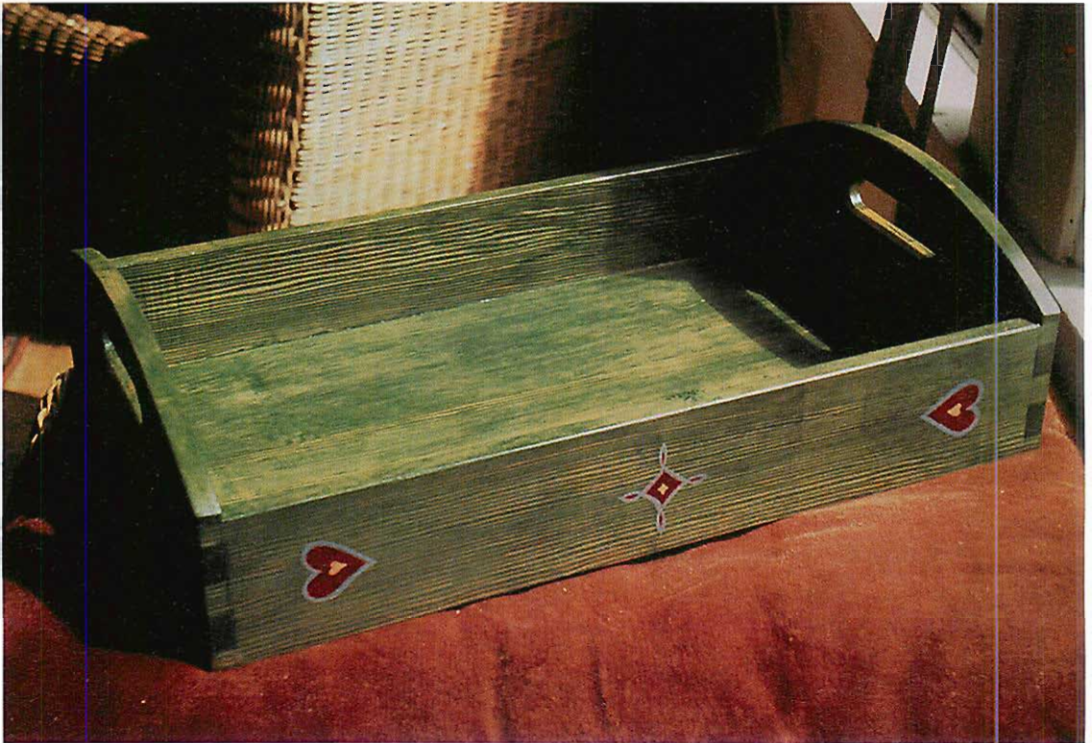
Pine tea tray with green French polish, and green oil pigment ad linseed oil, Christopher Alexander, 1972
